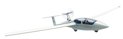
The ASK 21 Mi has a small engine delivering 41 kW. This is enough to allow the ASK21 Mi to take off eliminating the need for a tow aircraft and extending the cross-country capabilities. However, that does not mean this is a motor glider in the original sense of the word. The ASK21 Mi is classed as a 'motorized glider'. Like the ASK 21 it is a durable and robust aircraft, easy to fly and handle on the ground, you do not need any person to hold your wing.
